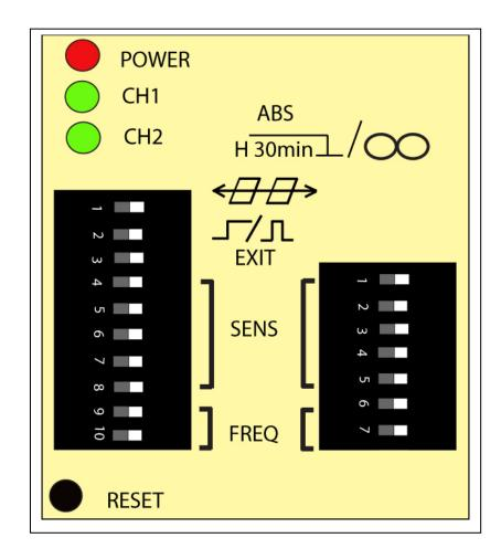
\* In the application, where two or more loop detectors and sensing loops have been installed, set one detector to high frequency and the other set to low frequency to minimize the effects of cross-talk between the two systems (The sensing loops and detectors should be positioned at least 2m apart).
